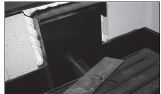
Air tube holds the air restricter.
