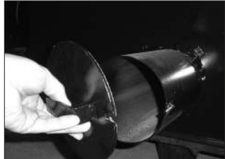
Removal of Ash Auger Tube Cover Plate
