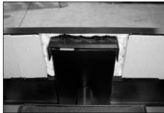
Air tube holds the air restricter.
