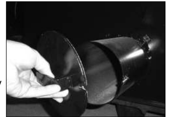
Removal of Ash Auger Tube Cover Plate
