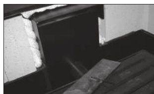
Air restrictor tube holds the air restrictor.
